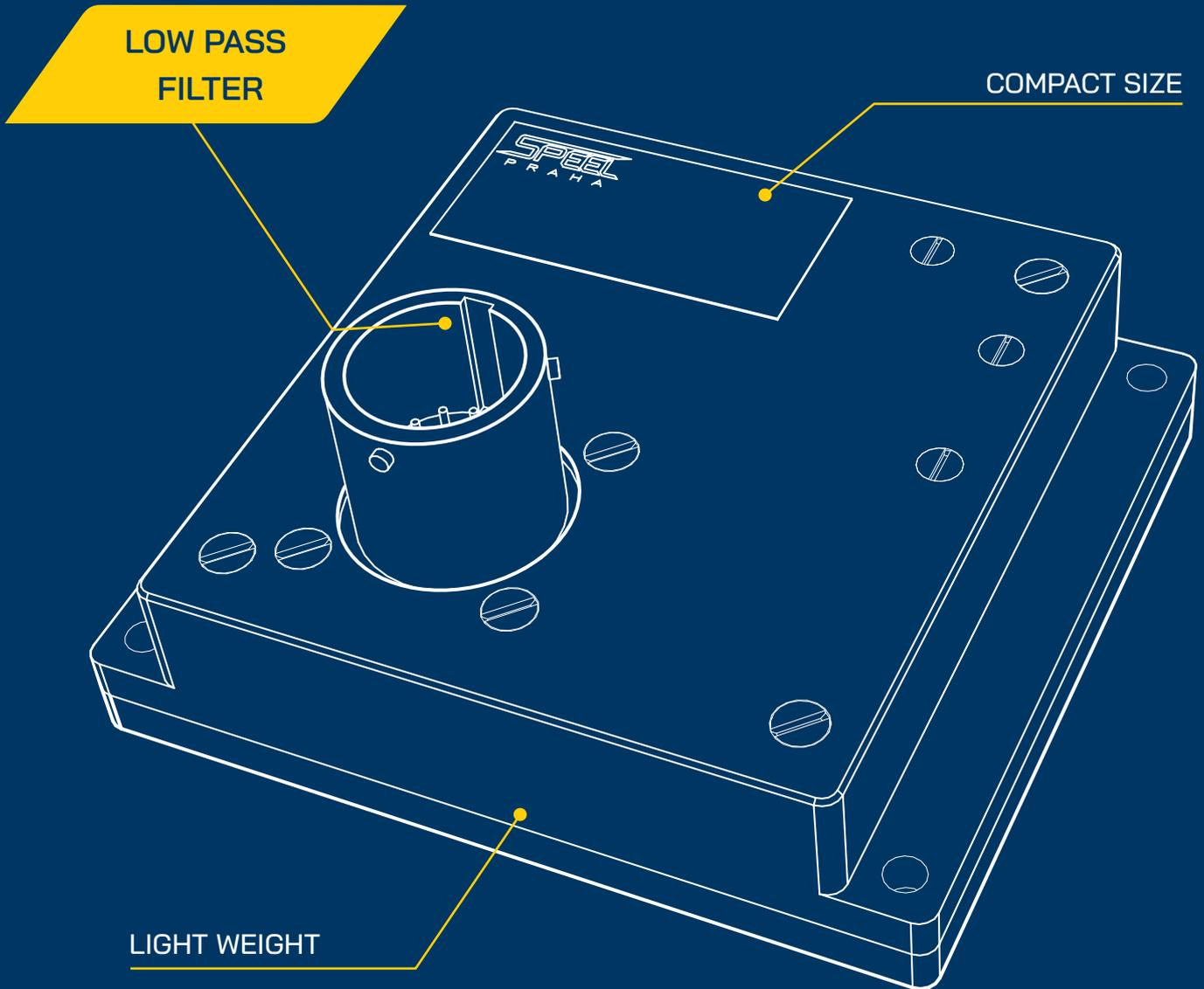
The 3-Axis Accelerometer, SACC 2640, senses accelerations of the aircraft in the longitudinal, lateral and vertical axes. It shall be placed close to the center of gravity of an aircraft. The output circuitry of the unit is equipped with low pass filters to avoid distortion of the signal caused by vibrations.
