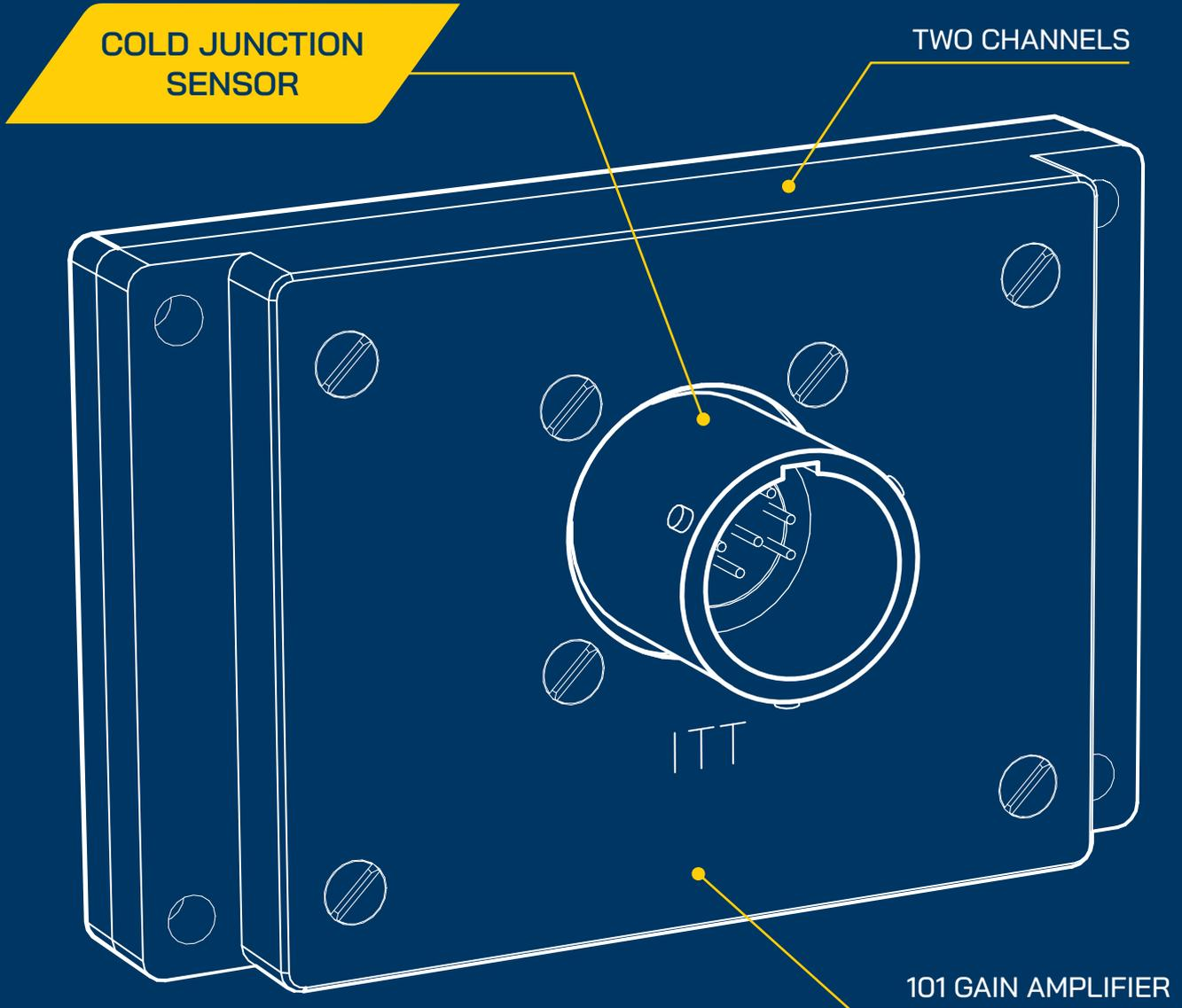
The Thermocouple Conditioner, ITT, houses circuitry for conditioning and amplifying two low voltage output signals of engine thermocouples with high gain. Inside the ITT, there is also a semiconductor thermometer sensing the temperature of thermocouples cold junction.
